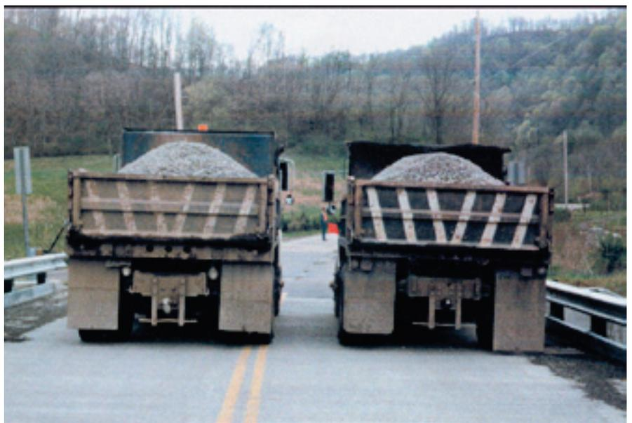
*W. Va. Dept. of Highways supplied test vehicles used to gather data for calculating distribution factors.*
